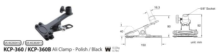
A handy multi-purpose steel clamp which features three attachment methods: a spring-tension with rubber feet protection clamp which has a clamping range of 5-40mm, a 5/8" female socket and a 5/8" stud so it can mount into a lighting stand, Convi Clamp, Super Viser or Grip Head to hold reflectors, gels, foam cores or a flash securely in the studio and on location.
