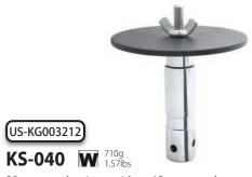
28 mm steel spigot with a 12cm round mounting plate fits into standard lighting stands or can convert a 28 mm receiver to a M10 thread with wing nut.
