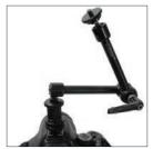
This adapter can fit on the hot shoe of most cameras. It has a 3/8" to 1/4" threaded stud and is used as a Monitor Bracket or anything else that has a 1/4" -20 receiver. Two large knurled locking nuts are quipped for easy adjustment of the tension. It comes with a 1/4"-20 double female barrel adapter as the standard accessory that makes the 1/4" -20 receiver is available.
