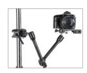
This camera bracket is designed for the Max Arm. Constructed with aluminum die-casting which makes it very lightweight and durable. In addition to a standard 1/4''-20 inch thread mount for a small camera, it also comes with a 1/4'' to 3/8'' adaptor to accept different sizes of thread mounts. There are four 3/8" female sockets available on the bracket that can connect two max arms from each side giving it the most stability. The 7mm female socket is also built for an umbrella reflector.
