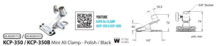
A compact clamp with 35mm clamping range similar to the Ali clamp but smaller. One of the most useful tools for a photographer, it can mount to the top of any lighting stand with a 5/8" socket or stud to hold props, reflectors and background drops or clip a small light fixture for tabletop shooting.
