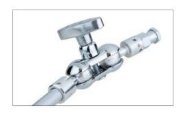
Articulated arm is used to lock and hold small lighting and effects in accurate position. The end socket is a 5/8" baby pin on the outside which can hold a small lighting fixture. The inside is a 3/8"-16 thread which will accept the standard dot and camera accessories.
