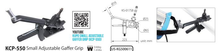
A quick mounting and multi-purpose clamp which will grip on flat or round surfaces. There is a variable tension rubberized control knob with a removable baby 5/8"(16mm) pin mounted in a female baby receiver in the handle and another 5/8"(16mm) pin mounted on the flat part of the jaw. The clamp works on diameters from 0.63-2.36" (16-60mm).
