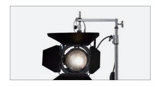
The 380mm Baby Offset Arm with two baby pins and one baby receiver, mounts on a baby stand where a light cannot be placed as close as desired to a subject or if you need to come over the top of the set to hide the stand behind a set wall. Caution: When offsetting a light it also offsets the weight, and it is necessary to place a sandbag or counterweight to prevent the tipping of the stand.
