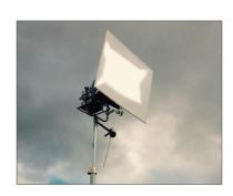
Kupo butterfly frames are made of heavy duty 30mm square section aluminum tubes, which can be easily locked together and disassembled for storage and transportation. Ear type frame supporters (or Stud type with wire for 20' x 20') are provided for mounting the buttery frame on the stands allowing for a stable frame for silks, scrims, etc.
