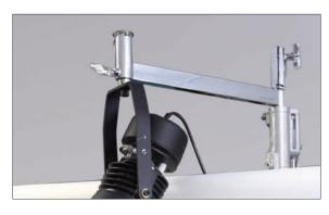
The 470mm Junior Offset Arm with a junior pin and receiver, can offset a large light fixture from its stand. It mounts to a stand with a junior pin top and with a junior receiver it allows a light to be mounted either over or under (a safety linchpin is attached). An additional junior receiver is welded for an extra lighting fixture or an umbrella while working on a rainy day.
