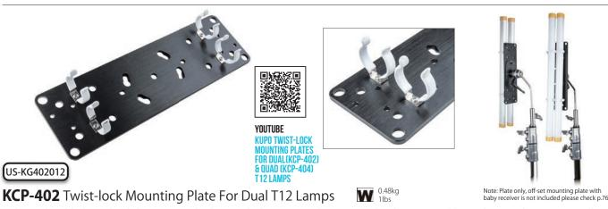
Lightweight & black anodized aluminum made, the twist-lock mounting plate equipped with two pair rubberized spring clips (KCP-401) allows it to mount 2 Kinof flo Lamp or T12 lamp. The plate comes with 4 pairs dia. 3/8" hole for fastening with cheese plate. The rest holes on each corner are for connecting and safeties. Size: 330 x 100mm.
