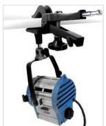
A quick mounting and multi-purpose clamp which will grip on flat or round surfaces. There is a variable tension control knob with a removable baby 5/8"(16mm) pin mounted in a female baby receiver in the handle and another 5/8"(16mm) pin mounted on the flat part of the jaw. The clamp works on diameters from 0.63-2.36"(16-60mm).
